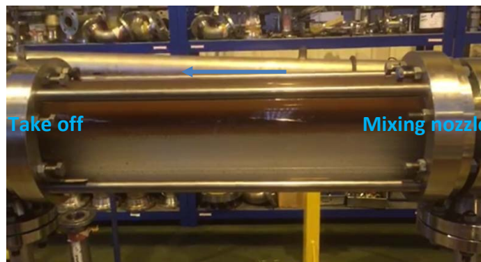
Figure 7: Picture of transparent test section
